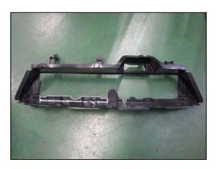
(2) Install the modified radiator air guide to the vehicle.
