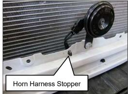
(2) Install the Oil Cooler Bracket No.2 to the hole the horn harness stopper was removed using the following provided parts as shown in the diagram on the right.
