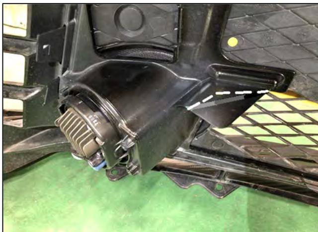
(9) Secure the wires shown in the diagrams below using the provided Tie Wrap S.
