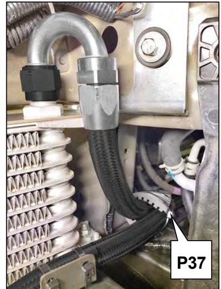
(19) Connect the Oil Cooler Hoses to the Oil Filter Mount.
