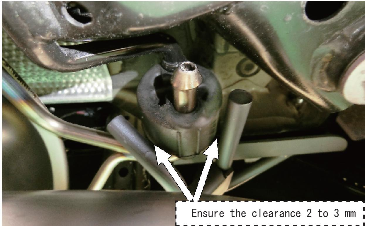
【 Fig. 3: Clearance between bracket and bumper 】
