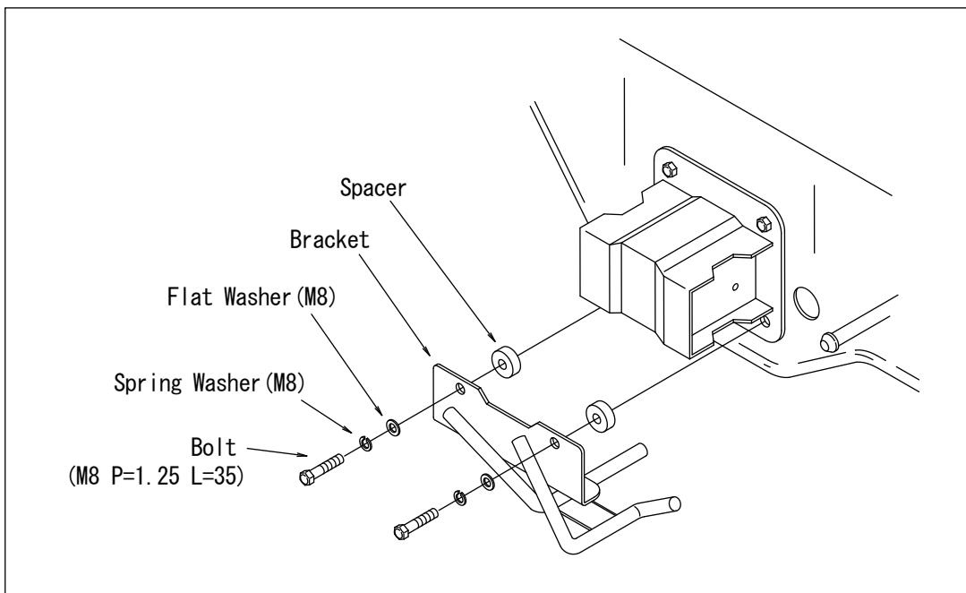
【 Fig. 2: Bracket installation figure 】
