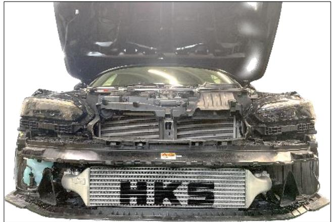
Use the removed ① bolt x 4, ② stay x 2, and ③ bolt x 2.
