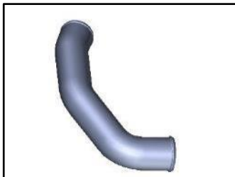
P4: Intercooler outlet pipe No.2
