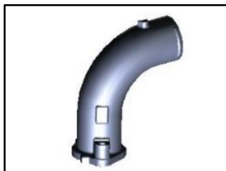
P2:Intercooler inlet pipe No.2
