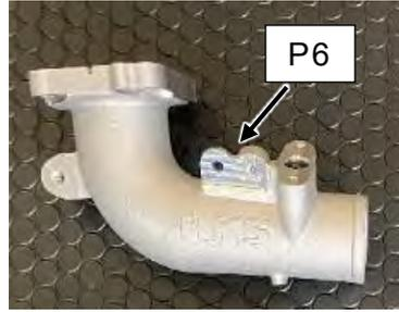
Remove the pressure sensor from the air tube assembly and attach it to the outlet pipe 2.
