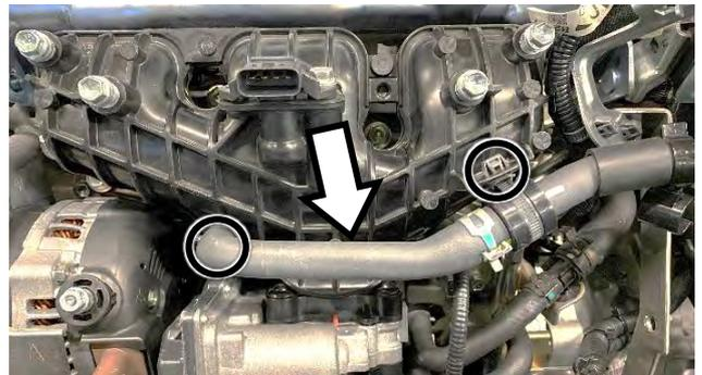
Remove the 2 bolts and 2 nuts, and remove the intake manifold.
