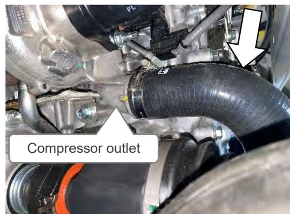
● Installation of outlet pipe 2
