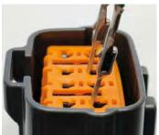
Use a precision screwdriver (-) to lift the retainer and release the lock.
