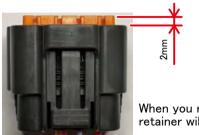
When you remove the lock, the retainer will pop out about 2mm.
