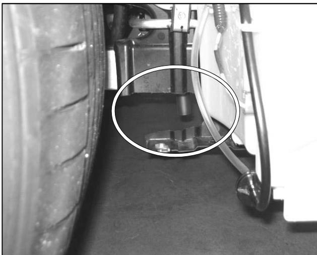
Cut the circled portion so Hose Assembly No.1 does not come in contact with.
