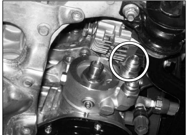
Adjust the clearance between the alternator and Oil Filter Mount assembly fitting.
