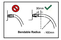
(4) When using a hose in a straight line in high-pressure areas, leave some slack in the hose. The length of the hose changes when pressurized, so leave some slack in the hose to compensate for this and avoid applying excess tension to it.
