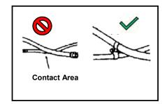
(3) The hose is easily deformed by twisting or excessive bending, so make sure that the hose is not bent less than the minimum bending radius (100 mm).
