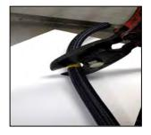
(2) Twist the hose while pushing it into the socket.
