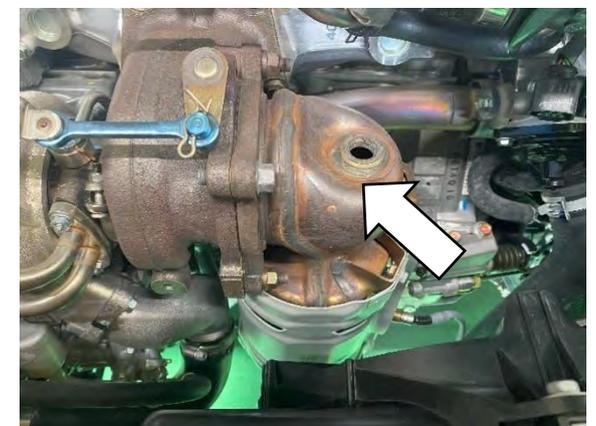
●Install the Heat Shield Plate and LAF Sensor.
