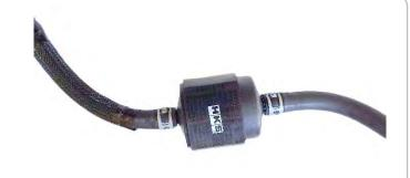
• Attach Oil Hose cut to 135 mm to Pump.
