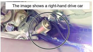
Place Pump on top of Suspension Member through Transfer Case and between Transfer Case and Suspension Member.
