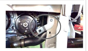
Connect Cooler Pipe to Oil Hose. Install Oil Hose according to the following instructions.
