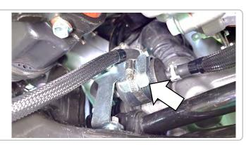
• Attach a 190mm Oil Hose to Transfer Drain.
