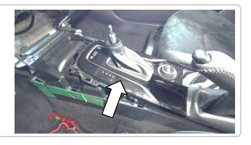
• Remove Parking Brake Hole Cover SUB-ASSY.
