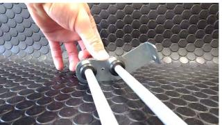
Attach Cooler Pipe assembly to Pop Nut installed on Reinforcement..
