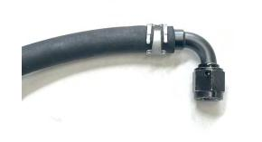
Secure Braided Tubing tightly to Oil Hose before securing it with vinyl tape.
