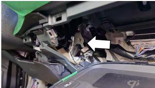
Power the Pump Controller from the floor wire to the Instrument Panel Wire #28.
