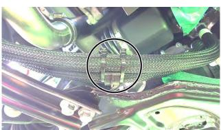
Tie the two hoses to the Intercooler Piping Bracket with tie wrap.
