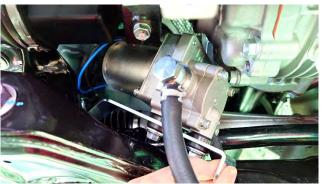
Temporarily fix Pump Bracket.
