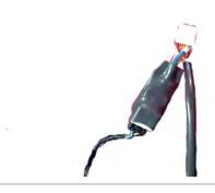
• Put together the excess wiring on the battery side.
