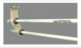
Install Cooler Bracket. Attach Cooler Brackets L and R, which have just been attached, so that they are sandwiched between the two brackets.
