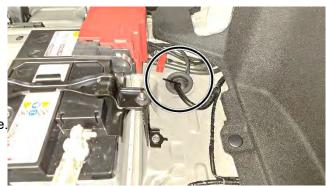
Secure the wiring in three places with Tie Wrap Base.
