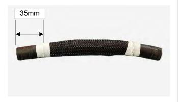
Cut Oil Hose to 135 mm (±3 mm) and install Pump Banjo Ø16.
