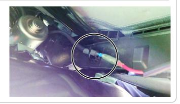
Remove paint from the pump ground terminal area in order to attach the ground terminal to the bolt on the vehicle body side of the battery wiring fixing bracket.
