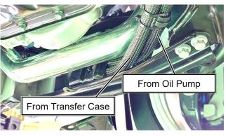
③Fix the 1170 mm Oil Hose connected to Transfer Case with Hose Clamp of Hose Bracket No. 2.
