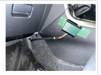
• Connect the Stag Terminal on the Main Harness to the Ground point.
