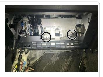
The red wiring of Connector A74 and the red wiring of the Main Harness are connected with a Splice and insulated with Vinyl tape.
