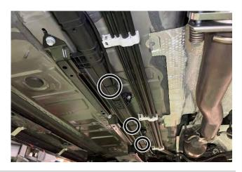
Secure the wiring in the Tie Wrap Base and Tie Wrap Medium.
