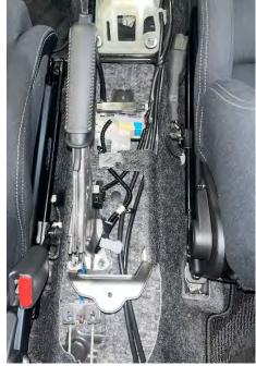
Secure the wiring in three places in the Tie Wrap.
