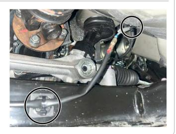
• Wire the Connector side of the Pump Harness room.
