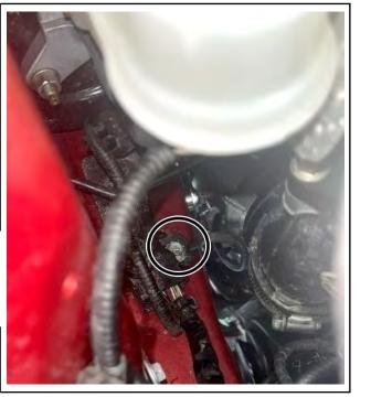
Install the Radiator Reserve Tank Assembly in the reverse of the procedure in which it was removed.
