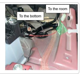
• Wire the Bullet Terminal side of the Pump Harness underneath.
