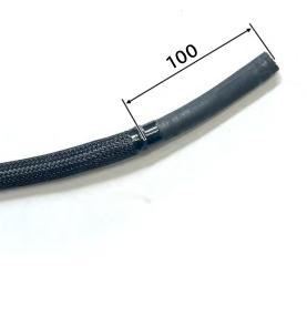
• Attach the Oil Hose to the Oil Pump.
