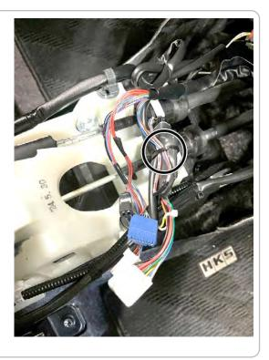
• Connect the Coupler of the Main Harness and the Select Switch.
