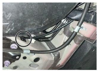
Secure the wiring in three places in the Tie Wrap.
