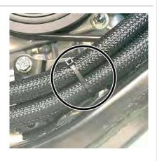
Before and after the clamping, tie the two oil hoses with Tie Wraps. Adjust the Hose Bracket No. 1 so that the Hose and Frame do not come into contact, and tighten the Cap Bolt.
