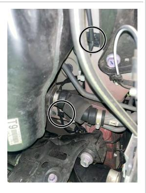
Secure the wiring in the Tie Wrap Base and Tie Wrap.
