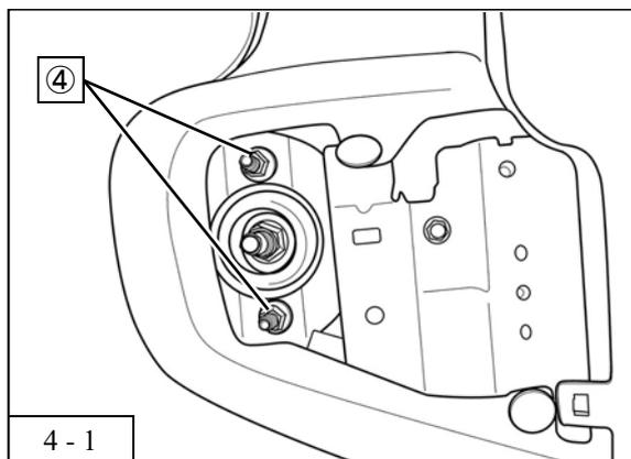
1. Install the provided rear suspension assy to the vehicle using the upper rear suspension assy installation nuts ④ .
