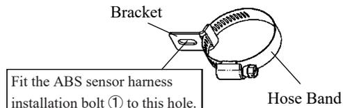
After installing the universal bracket, make sure tension is not applied to the ABS sensor harness when a steering wheel is turned and/or suspension is stroking.
