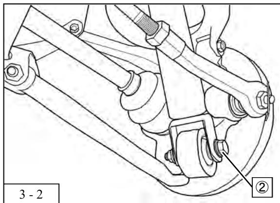
4. Remove the bolt and nut from the lower rear suspension assy (2).
