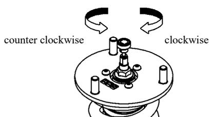
Turn the dial attached on the top of each shock absorber
