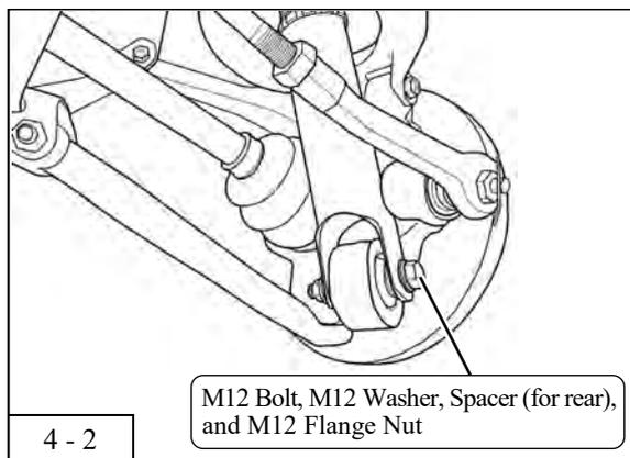
2. Install the provided M12 bolt, washer, spacer (for rear) and M12 flange nut.
