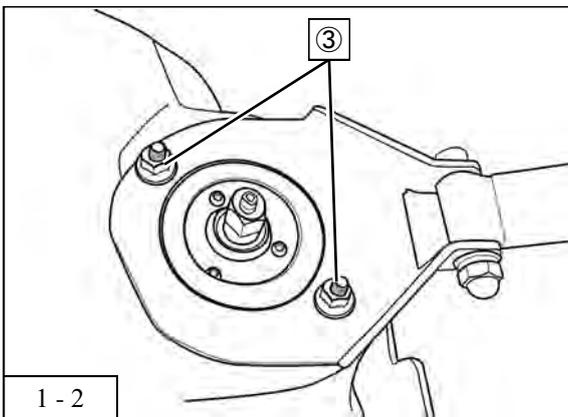
3. Remove the nuts from the upper front suspension assy ③.
