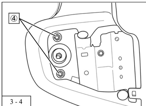
6. Remove the nuts from the upper rear suspension assy (4).
