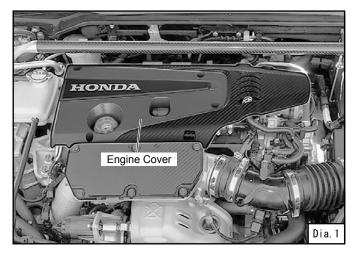
(2) Install the engine cover using M6-35 bolts. (Dia. 2) (Tightening torque: 14 N-m {1.43 kgf-m})
