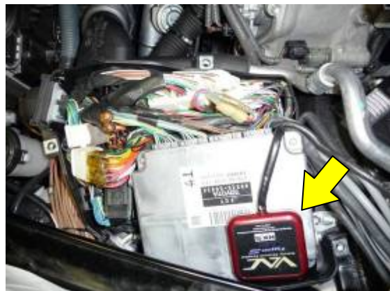
Mount the VAC using a double-sided tape.
