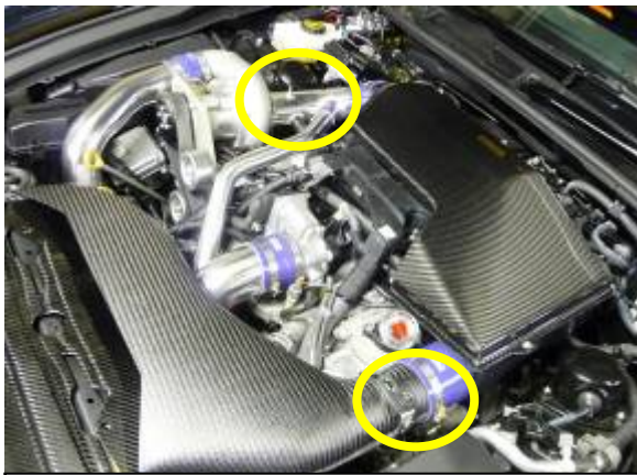
Insert the mounting rubbers to the mounting bolts. Install the Engine Cover.
