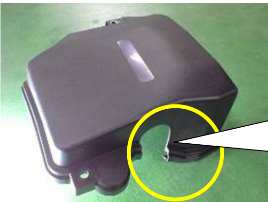
Modify the ECU box so the harness can be routed. Reinstall the box.
