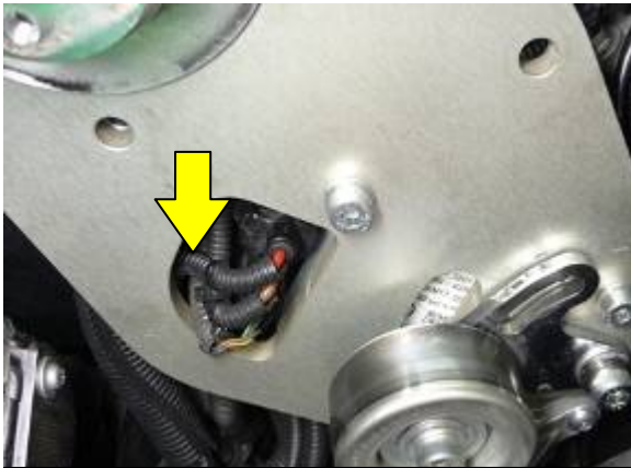
VTC harness can get out of the opening for the bracket.
