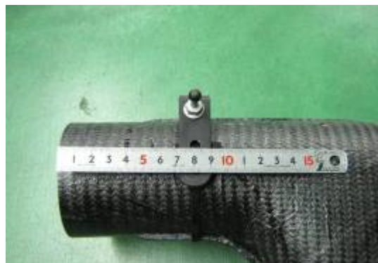
Affix the sponge sheet to the duct side. Install the bracket.
