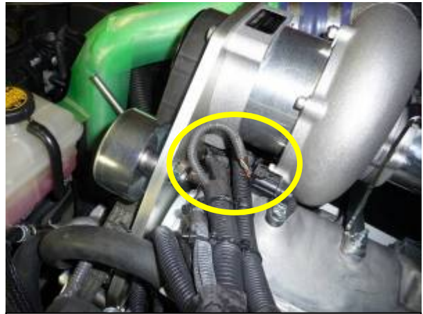
Route the harness between the GTS8550 and cylinder head.
