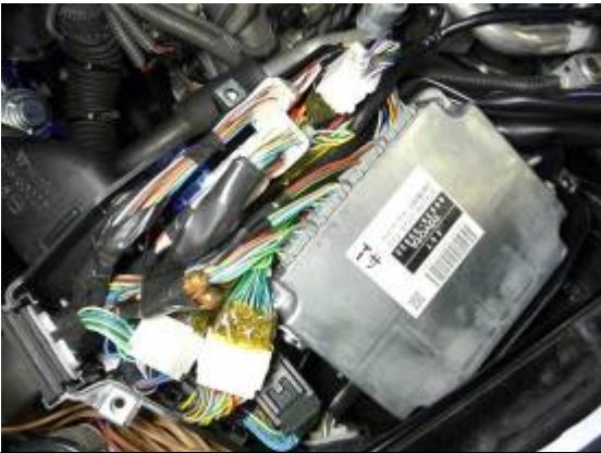
After installing the F-CON Harness, connect the ECT connector.
