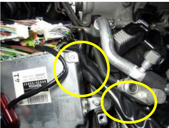
Route the F-CON Harness as shown above.
