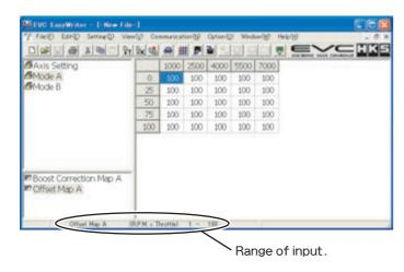
This offset is used to make fine adjustments to the set boost in Mode A/B relative to throttle position, RPM, or speed. For example, if the set boost for Mode A is 120%, and Boost Correction A is 20%, then the target will be 140%. The boost will increase if the set value is increased and the boost will decrease if the set value is decreased regardless of bypass type being used.
