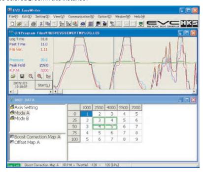
Make sure the correct data is selected. This function will execute even for log data that is not recorded in the display window.
