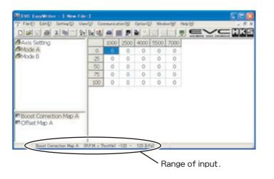
Correction will be performed according to the boost correction value of the throttle position, RPM, and speed in addition to the set boost in Mode A/B. For example, if the set boost for Mode A is 100kPa, and Boost Correction A is 10kPa, then the target will be 110kPa.
